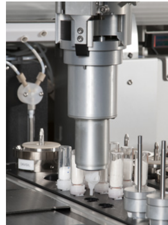
SV dispensers use vibration for precise delivery
