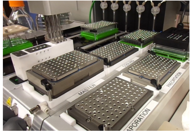
Heated filter block on temperature controlled station
