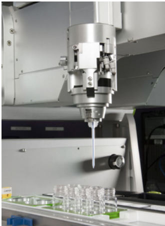
Viscous liquid dispenser handles up to 1000 cP
