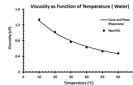
Figure 1. Comparison of NeoVISC™ to Conventional Rheometer
