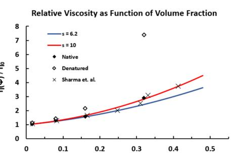
Figure 4. Comparison of NeoVISC BSA Viscosity to Colloidal Rheology Models
