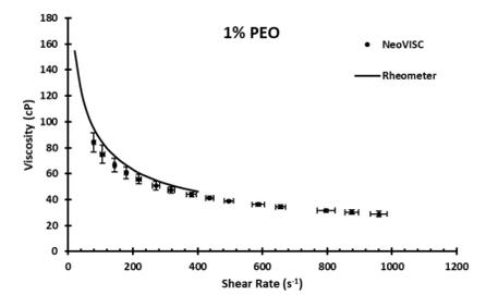
Figure 2. True Viscosity as Function of Shear Rate for Non-Newtonian Fluid
