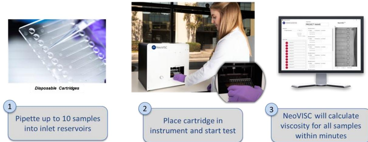
**Figure 1. NeoVISC™ workflow.** To perform a NeoVISC™ measurement, user pipettes samples into the cartridge, places the cartridge in the instrument, and begins the test via the proprietary user interface.
